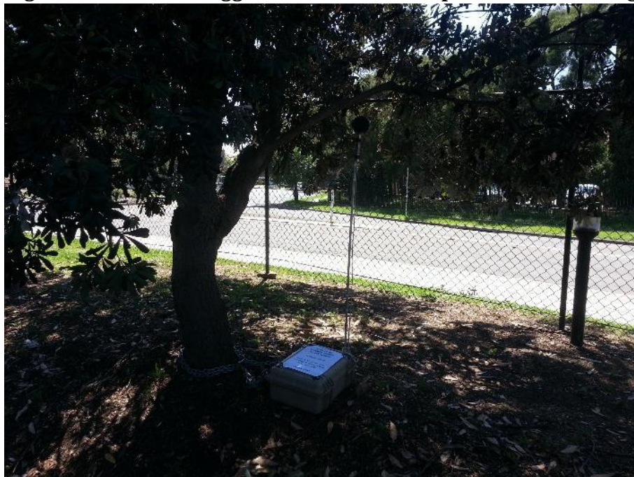
Figure 10-1 Noise Logger Installed near Shepherd Street frontage
