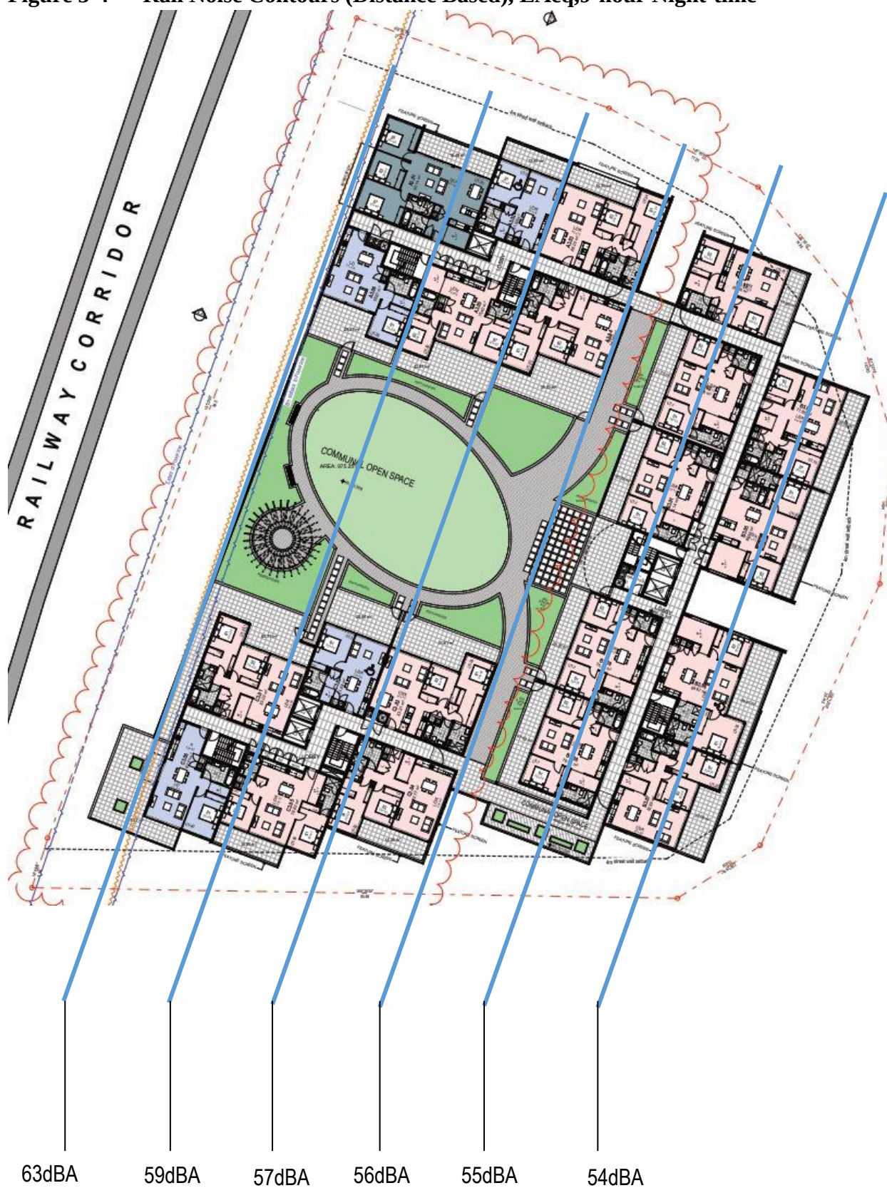
Figure 3-4 Rail Noise Contours (Distance Based), LAeq,9-hour Night-time
