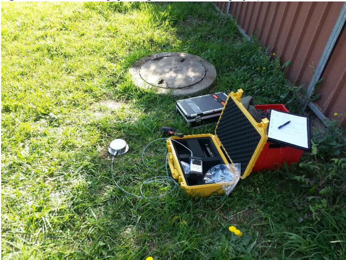
Figure 6-3 Vibration Equipment (photo from another project)
